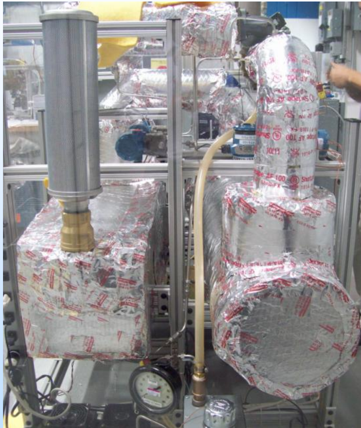
Test Rig for Blower Performance and Endurance Test
